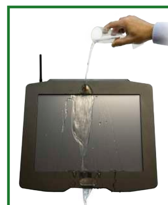
Water and Dust Proof Test IP66
